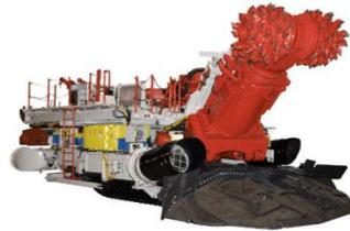
**Rozadora de Roca Rc < 100MPa**
